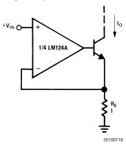
$I_O = 1$  amp/volt  $V_{IN}$ (Increase  $R_E$  for  $I_o$  small)
