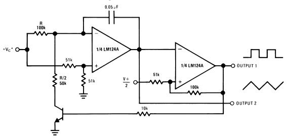
\*Wide control voltage range: 0  $V_{DC} \le V_C \le 2$  (V<sup>+</sup> -1.5  $V_{DC}$ )
