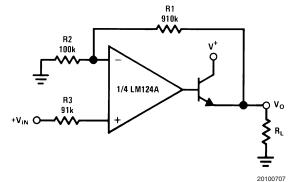
$V_0 = 0 \ V_{DC} \text{ for } V_{IN} = 0 \ V_{DC}$ A<sub>V</sub> = 10
